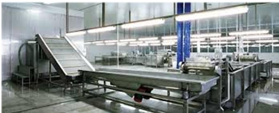
Figure 11 - Fluidized IQF Freezer
